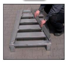
Insert safetywedge diagonal into the pallet deck
