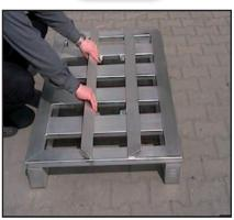
To take off or to move the wedges please fold up the wedges (remove them)- now the wedges are flexible for a new width or removable
