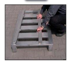
Press down to fix the safetywedges
